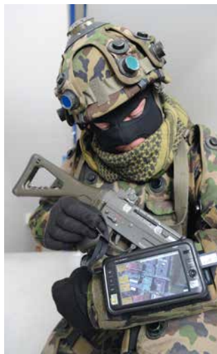
Indoor Localisation System with wrist-mounted display
