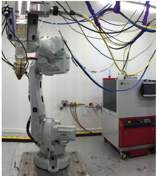
*The R&D project in operation, showing the Laserline system with the uniquely designed nozzle mounted on a robotic arm.*
